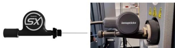
Figure 2. IonOpticks Aurora SX nanoflow columns connected to the OptiFlow TurboV ion source on the ZenoTOF 7600 system.
