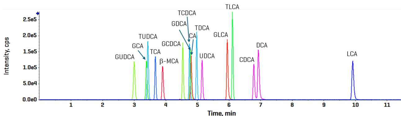
**Figure 3. Elution profile of targeted bile acids using CID-based fragmentation in the negative ion mode.** The 50 nM standard was injected and analyzed using the sMRM scan mode. Total run time was 17 min.
