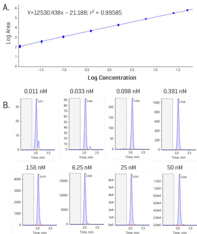
**Figure 4. Example internal standard curve with representative peaks for GUDCA. [A]** Internal standard curve for GUDCA from 0.011 to 50 nM. **[B]** Example chromatograms at each concentration level of the curve; blank region highlighted in grey.
