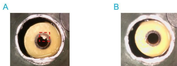
Figure 6. The bottom-up view of the OPI port after running plate 249. Images show the OPI from (A) the baseline study without the OPI port wash and (B) the study with OPI port wash performed after every 384 ejections. Both images were captured after running plate 249. The deposit inside the electrode assembly was clearly visible without the OPI port wash (red dashed rectangle), whereas no distinct foreign components were observed with the OPI port wash.
