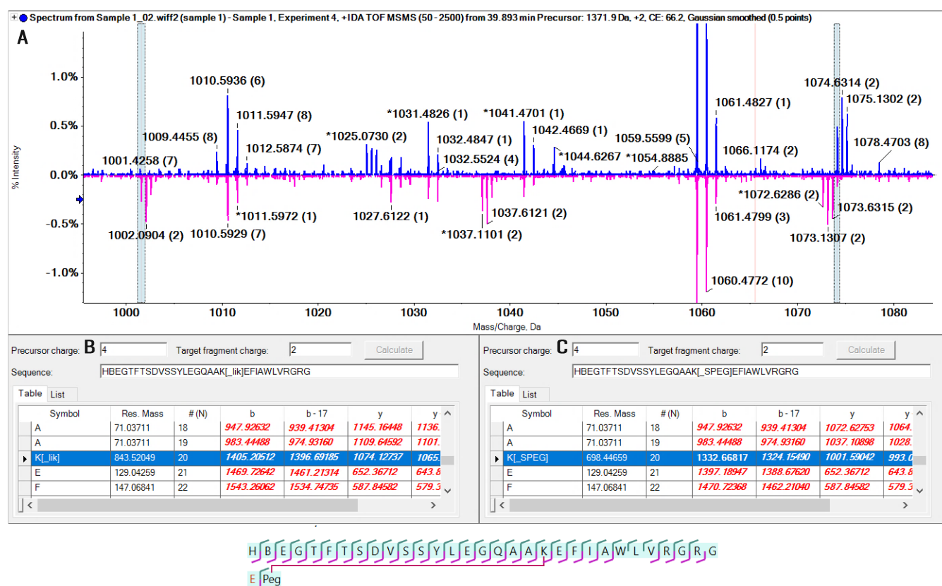
Figure 7. Characterization of linker loss at amino acid K (position 20 from the N-terminal). The top panel in the mirror plot shows conventional semaglutide fragment ions with the y12 ion as 1074.12 Da, while the bottom panel shows the y12 ion as 1001.59 Da, confirming a loss of a PEG molecule with a mass of 145 Da (A). The theoretical fragment masses of both species are shown at the bottom, highlighting changes in the mass of the linker attached [ lik : full linker, SPEG : truncated monoPEG linker, B: aminobutyric acid] (B-C).
