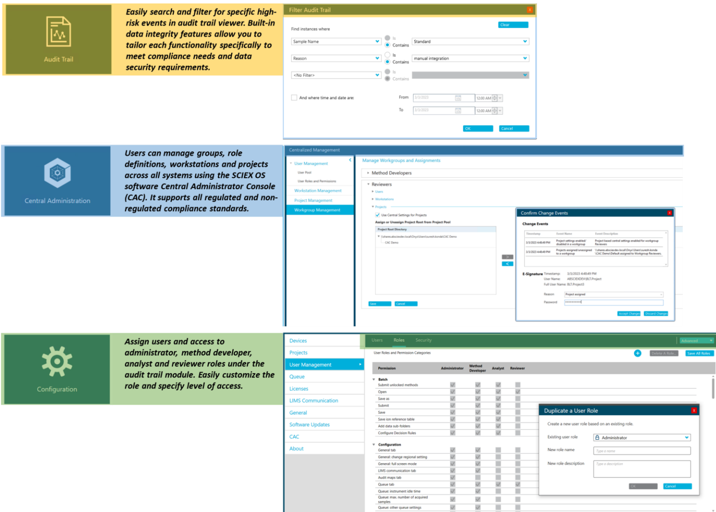
Figure 3. Features of the SCIEX OS software for monitoring user access and evaluating the audit trail. The audit trail view allows users to filter for high-risk events easily and enables data integrity features to meet compliance requirements. The software features a Central Administrator Console (CAC) to manage users and groups, role definitions, workstations and projects across all systems. The CAC feature supports both regulated and non-regulated compliance standards. The configuration module enables users to quickly set up roles and levels of access for the administrator, method developer, analyst and reviewer levels.
