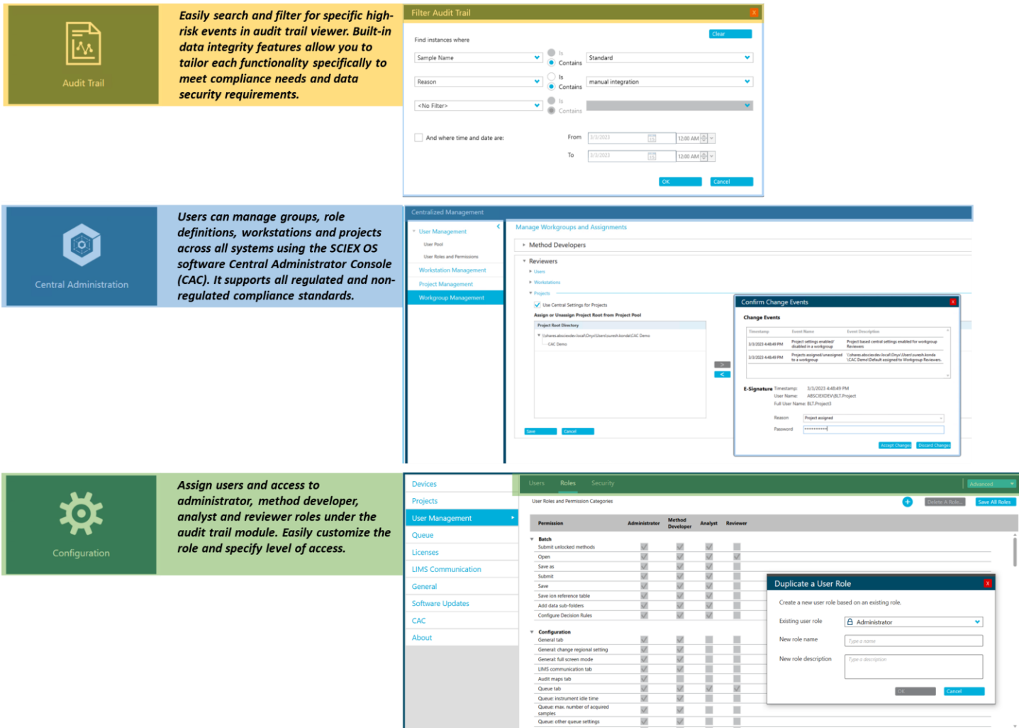
Figure 5. Features of the SCIEX OS software for monitoring user access and evaluating the audit trail. The audit trail view allows users to filter for high-risk events easily and enables data integrity features to meet compliance requirements. The software features a Central Administrator Console (CAC) to manage users and groups, role definitions, workstations and projects across all systems. The CAC feature supports both regulated and non-regulated compliance standards. The configuration module enables users to quickly set up roles and levels of access for the administrator, method developer, analyst and reviewer levels.
