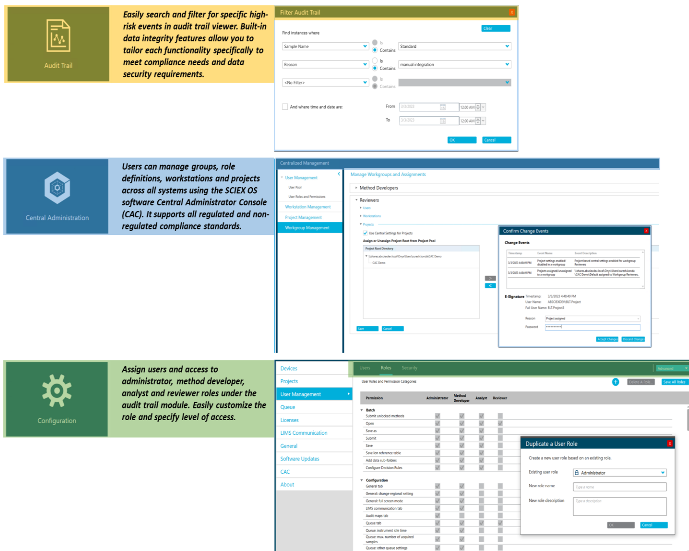
Figure 4. Features of SCIEX OS software for monitoring user access and evaluating the audit trail. The audit trail view allows users to filter for high-risk events easily and enables data integrity features to meet compliance requirements. The software features a Central Administrator Console (CAC) to manage users and groups, role definitions, workstations and projects across all systems. The CAC feature supports both regulated and non-regulated compliance standards. The configuration module enables users to quickly set up roles and levels of access for the administrator, method developer, analyst and reviewer levels.
