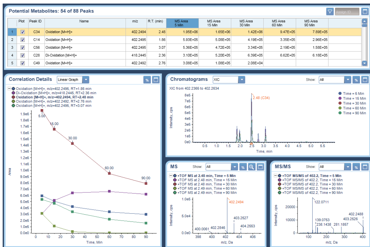
Figure 6. MetabolitePilot 2.0 Software Correlation Workspace. An example correlation plot for the oxidized metabolites of buspirone from 5 to 90 min incubation time points is shown. The correlation is shown in a linear plot with overlays of chromatographic, MS, and MS/MS data, bar graph and table views are also available in this correlation workspace.
