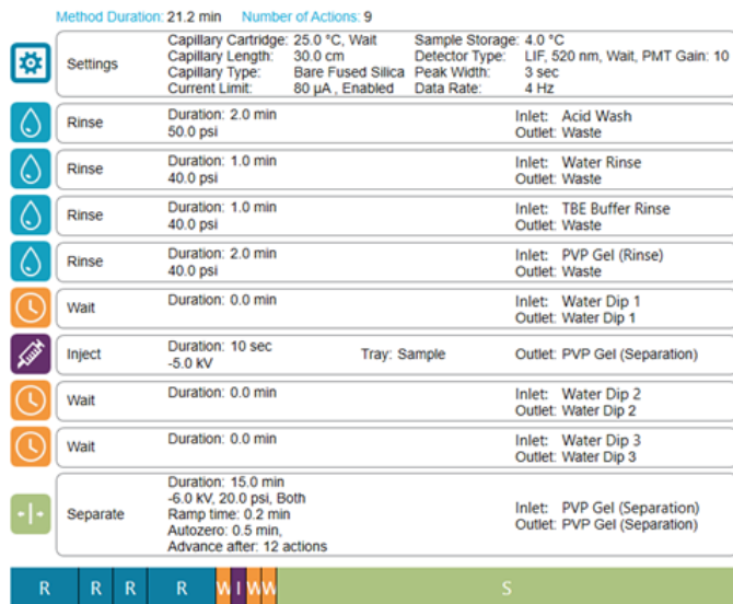
Figure 4. Settings for sample separation method as shown on the BioPhase software.
