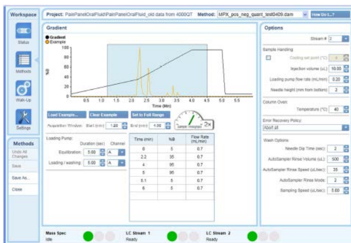
Figure 2. MPX chromatographic method. By using a multiplexed LC strategy with MPX, the injection-to-injection time can be shortened to 3.5 min.
