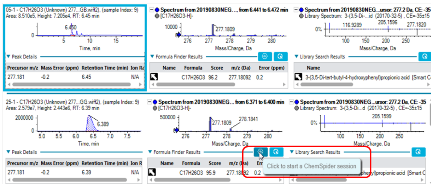
Figure 6. SCIEX OS software can be directly linked to the ChemSpider database to explore potential candidate structures for m/z features.
