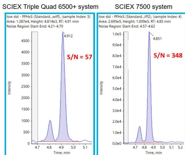
**Figure 1. MRM peaks for perfluorohexanesulfonic acid (PFHxS).** The SCIEX 7500 system data (right) shows a 7.1x increase in S/N compared with the SCIEX Triple Quad 6500+ system data (left). Note: gray shaded areas represent the noise region used for the S/N calculation.
