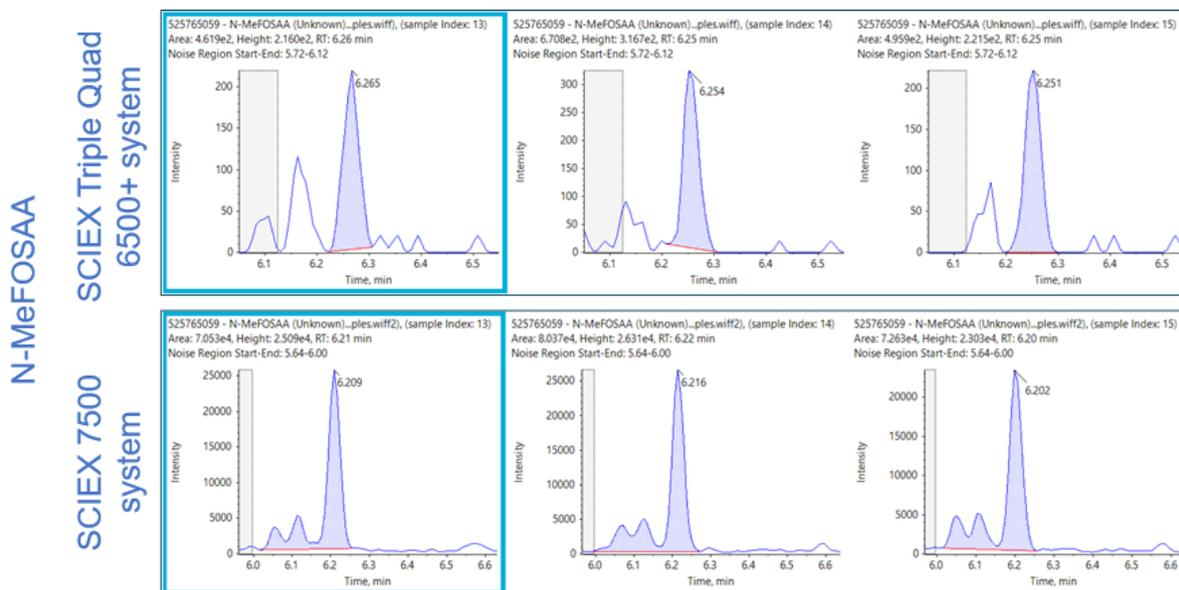
**Figure 7. Quantification of N-methylperfluorooctane sulfonamidoacetic acid (MeFOSAA) in a surface water sample.** Triplicate analysis comparing the SCIEX Triple Quad 6500+ system (top) and the SCIEX 7500 system (bottom). The higher S/N observed with the SCIEX 7500 system leads to the detection of low-level isomers in the analysis.
