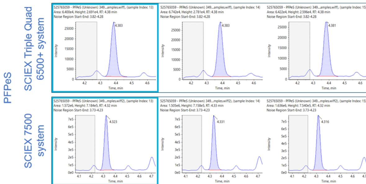
**Figure 6. Quantification of perfluoropentane sulfonic acid (PFPeS) in a surface water sample.** Triplicate analysis comparing the SCIEX Triple Quad 6500+ system (top) and the SCIEX 7500 system (bottom). The higher S/N observed with the SCIEX 7500 system leads to higher precision and confidence in the analysis.
