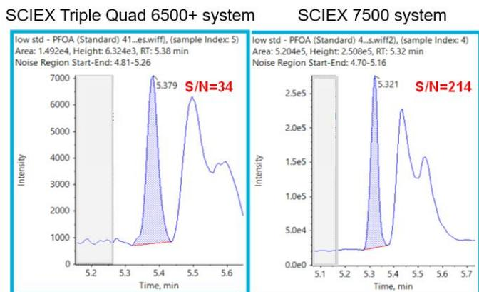
**Figure 3. MRM peaks for perfluorooctanoic acid (PFOA).** The SCIEX 7500 system data (right) shows a 13.5x increased S/N compared with the SCIEX Triple Quad 6500+ system data (left). Note: gray shaded areas represent the noise region used for the S/N algorithm.
