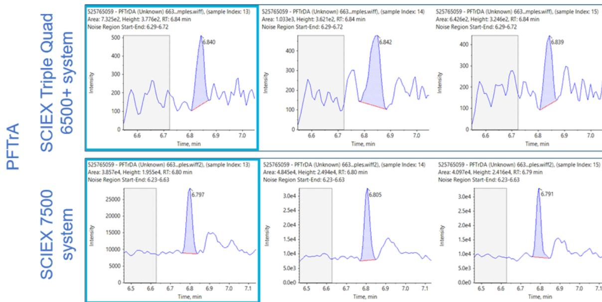
**Figure 8. Quantification of perfluorotridecanoic acid (PFTrA) in a surface water sample.** Triplicate analysis comparing the SCIEX Triple Quad 6500+ system (top) and the SCIEX 7500 system (bottom). The higher S/N observed with the SCIEX 7500 system leads to the detection of unexpected low-level analytes.
