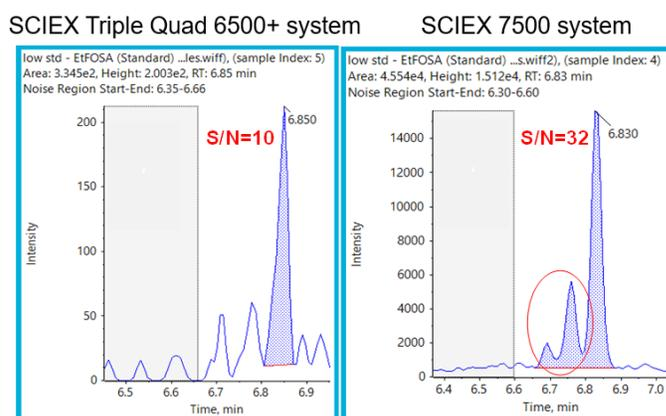
**Figure 4. MRM peaks for N-ethyl perfluorooctane sulfonamide (EtFOSA).** The SCIEX 7500 system data (right) shows a 3.8x increased S/N compared with the SCIEX Triple Quad 6500+ system data (left). The increased S/N enables quantification of important lower-level EtFOSA isomers (red circle) that are missed using the SCIEX Triple Quad 6500+ system. Note: gray shaded areas represent the noise region used for the S/N algorithm.
