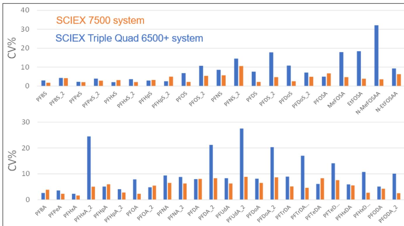
**Figure 5. Precision for 5 replicate injections of the low-level standard.** The SCIEX 7500 system had CVs of <10% for all PFAS transitions (orange bars) while the CVs for the SCIEX Triple Quad 6500+ system were generally under 20%, but with some outliers ranging up to 30% (blue bars).
