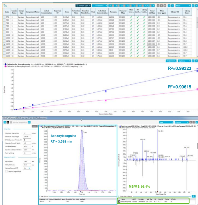
Figure 1. Obtain Both High Quality Quantitation with Confident Identification in a Single Workflow. Quantitation of Benzoylcegnine using MRM HR Workflow with the simultaneous generation of full scan MS/MS data provided 4 orders of linear dynamic range (top) for quantitation and a confidence identification using ion ratio computation (bottom left) and automatic library matching (bottom right).
