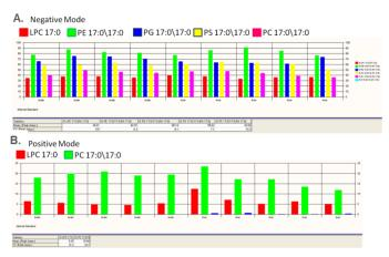
Figure 8: Lipid class internal standards can be reviewed for sensitivity and reproducibility in LipidView software. Phosphoglycerolipid internal standards detected in negative mode [A] and positive mode [B] are shown with calculated %CV across all samples.
