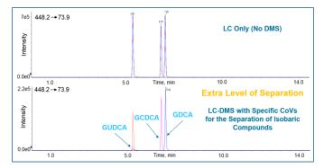
On-Column SelexION Separation of GDCA, GCDA and GUDCA. Without DMS (upper pane), only LC separation of these bile acids is possible. For all three isomeric compounds, the same transition is used (448.2 -> 73.9). Adding the compound-specific Compensation Voltage (CoV) to the SRM table of transitions allows only the isomer with the corresponding CoV to enter the MS for detection hence separating different isomers (lower pane) allowing more confident detection.
