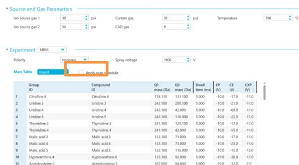
The screenshot shows the 'Experiment' section of the SCIEX OS software. The 'Polarity' dropdown menu is open, and 'Negative' is selected, highlighted by an orange box. The 'Mass Table' is visible below, showing the same 11 metabolites as in Figure 5-1.
