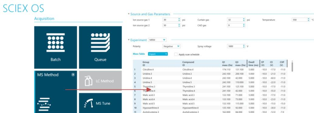
The screenshot displays the SCIEX OS software interface. On the left, the 'Acquisition' panel is visible with buttons for 'Batch', 'Queue', 'MS Method', 'LC Method', and 'MS Tune'. The 'MS Method' dropdown menu is open, showing 'MRM' selected. The 'Experiment' section shows 'MRM' selected, 'Polarity' set to 'Negative', and 'Spray voltage' set to '1600' V. Below this is a 'Mass Table' with the following data:
