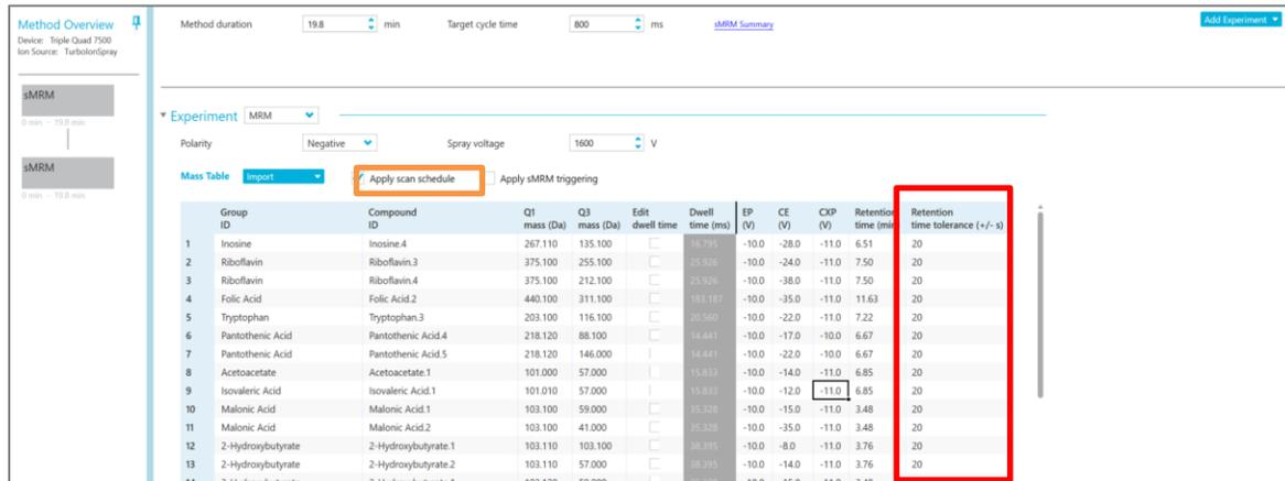
The screenshot shows the 'Method Overview' for a Triple Quad 7500 instrument. The 'Experiment' section is set to 'MRM' with a 'Negative' polarity and a 'Spray voltage' of 1600 V. The 'Mass Table' is set to 'Import' and the 'Apply scan schedule' checkbox is checked. The table below lists 14 compounds with their respective mass values and retention times. The 'Retention time tolerance (+/- s)' column is highlighted in red, showing a value of 20 for all entries.
