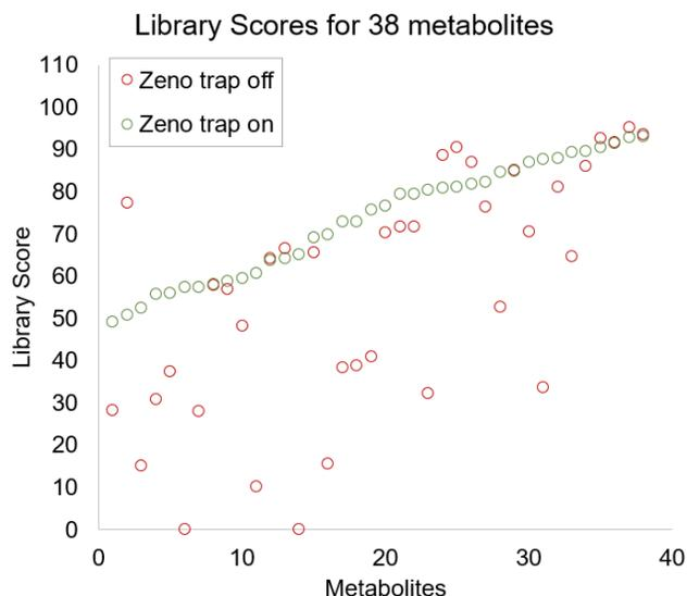
**Figure 1. Large sensitivity gains observed in Zeno MS/MS resulted in higher library scores.** Urine metabolites with library scores between 50 and 90 in the Zeno trap on data (green) were aligned with the Zeno trap off data (red). Library scores were typically higher in the Zeno trap on data, see Figure 4 for more details.
