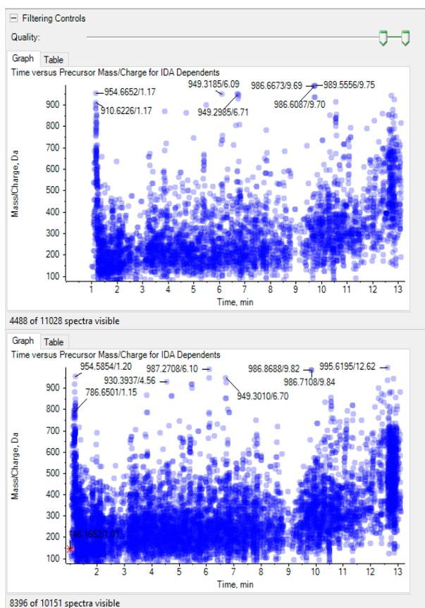
**Figure 2. Use of the Zeno trap greatly increases the spectral quality during data dependent acquisition.** MS/MS spectrum obtained with Zeno trap off (top panel) showed 40% of spectra (4488/11028) had a quality score  $\geq$  95. With Zeno trap turned on, (bottom panel) 83% of spectra 8396/10151) had a quality score  $\geq$  95. Data shown is for DDA collected on the ZDF male pooled sample.
