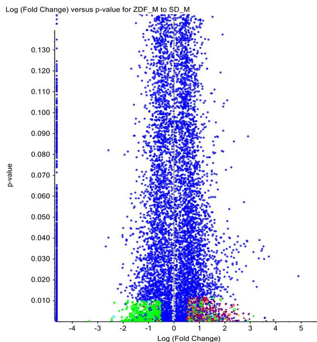
**Figure 5.** Detection of significant features from MS1 data. Significant features ( $p\text{-value} \leq 0.01$ ,  $\pm \text{Log fold change} \geq 0.5$ ) were selected from the MS1 peak processing in MarkerView software. An interest list of 4222 features was extracted and then processed using SCIEX OS software to identify the features.
