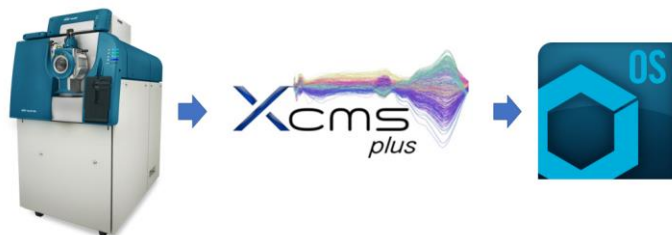
Figure 1. Workflow for metabolic profiling using the TripleTOF System. Data is taken from the TripleTOF 6600 System and processed through XCMS Plus software for feature finding. The metabolite identifications are confirmed by taking the metabolites of interest and passing them through the accurate mass metabolite library in SCIEX OS Software or MasterView™ Software.
