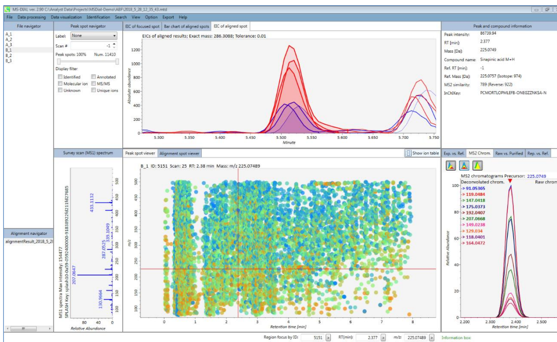
Figure 3. The MS-DIAL results window for easy data visualization. The graphical interface includes the File Navigator which shows the loaded files, while the Alignment Navigator shows the alignment results of the loaded files. The Peak Spot Navigator allows filtering of the results in several ways (identified peaks, annotated peaks, etc). The EIC Panel shows the extracted ion chromatograms of the spots highlighted in the Peak Spot Viewer where the color corresponds to the intensity. Lastly, the top panel shows Peak and Compound Information for an identification, and below are the aligned raw MS/MS chromatograms or the raw and purified product ion spectra.
