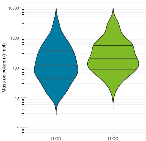
**Figure 6. Summary of observed quantification results.** The LLOQ and LLOD values were determined for the heavy labeled peptides in plasma. The median LLOQ was found to be 193 amol on column (green) and the median LLOD was 114 amol on column (blue).
