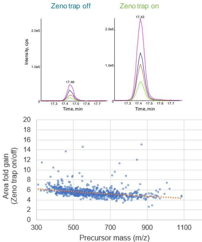
**Figure 1. Significant gains in peptide area with Zeno trap activated.** (Top) Example data of the sensitivity increases observed when the Zeno trap is activated are shown for ANT3.PFLVFIR, with a ~6x gain in peak area. (Bottom) A summary of the observed sensitivity gains for all 804 peptides is shown, plotted according to precursor mass. The average gain is 5.6-fold.
