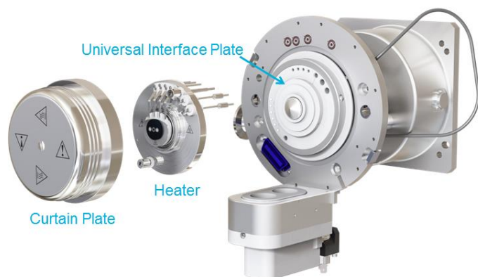
Figure 1. OptiFlow Interface for rapid switching between high flow and low flow sources. Easily switch between all front end operational modes in minutes, without having to break vacuum. For low flow applications, remove the high flow Curtain Plate, then install the nanoflow heater onto the Universal Interface Plate, and finally install the nanoflow Curtain Plate.
