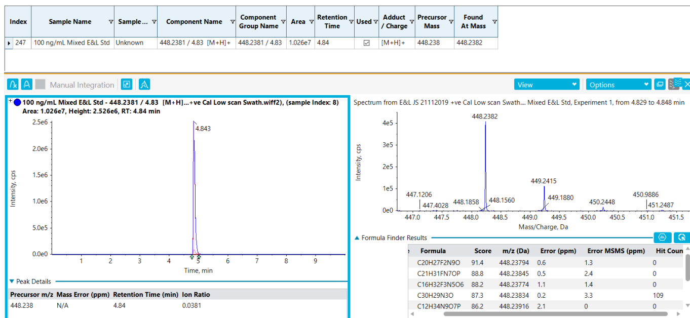
Figure 5. Formula Finder in SCIEX OS Software. First, a non-targeted peak finder is used to extract the MS and corresponding MS/MS data from the SWATH Acquisition data. Then Formula Finder is used to predict possible formulas based on precursor molecular weight and mass accuracy, the isotope pattern and the MS/MS fragmentation pattern. This provides a narrowed list of possibilities that can be further evaluated with ChemSpider.
