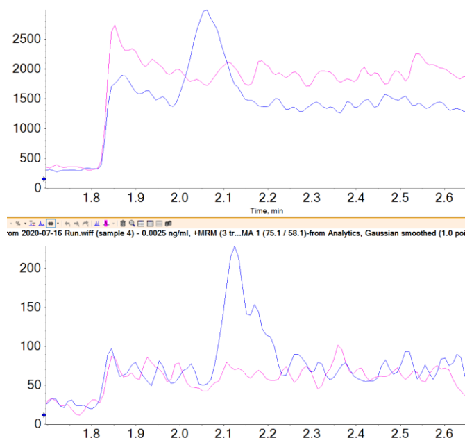
Figure 4. Significant reduction in background interferences. 2.5 ng/mL std, in Blue and blank in Pink, without (top) and with (bottom) SelexION Technology. While this point was visible without DMS, it was not reproducible enough to use for quantification. Note the solvent related background at 1.8 min when the divert valve switches inline.
