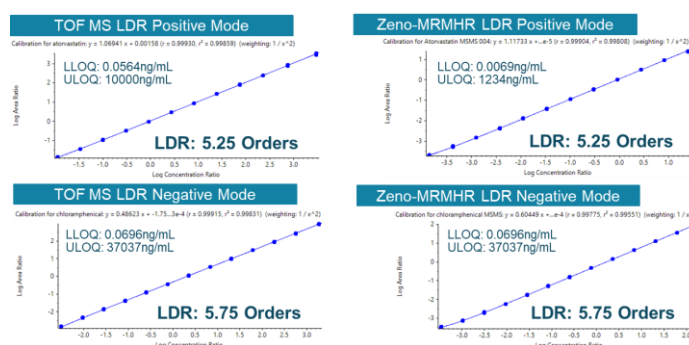
Figure 11: Linear dynamic range of the 4-channel NCP detector with ADC signal processing. Greater than 5 orders of inter-scan linear dynamic range can be achieved in both positive ion (top) and negative ion (bottom) modes, for both MS (left) and MS/MS (right) acquisitions.
