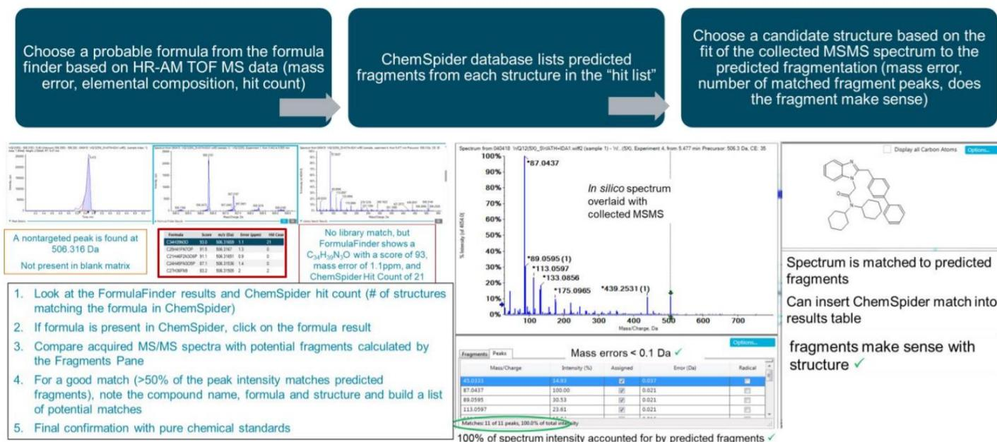
**Figure 1. Functionality in Analytics module links ChemSpider Database to FormulaFinder and experimentally derived MS/MS spectral data.** An unknown peak which does not have a library match, can still result in a FormulaFinder formula match with low mass error and ChemSpider hit count. ChemSpider can generate candidate structures for each formula with a matching of MS/MS spectra to predicted fragment ions.
