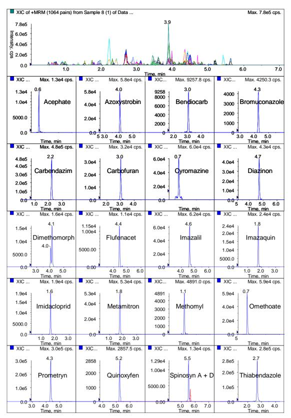
Figure 2. Pesticide Screening using 1064 Scheduled MRM<sup>™</sup> Algorithm transitions in less than 10 min (top) and extracted chromatograms of individual pesticides at a concentration of 1 ng/mL (bottom).
