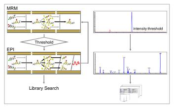
**Figure 1.** Setup of an Information Dependent Acquisition (IDA) experiment: A survey in Multiple Reaction Monitoring (MRM) screens for a multitude of targeted analytes with highest selectivity and sensitivity. The chromatographic signal above a specified threshold triggers automatically the Enhanced Product Ion (EPI) scanning. Acquired EPI spectra are searched against a mass spectral library for identification.
