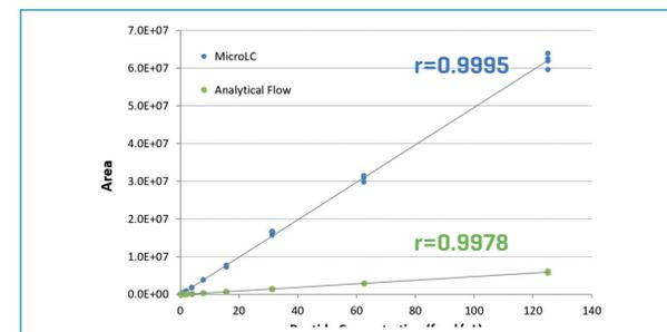
Calibration curves are shown for a synthetic peptide (VGNEIQYVALR) in diluted crashed plasma using microflow LC-MS at 3 µL/min and analytical flow LC-MS at 500 µL/min. LLOQ with microflow LC was 8x lower than what could be achieved with analytical flow LC-MS, and linearity was excellent for both flow rates.
