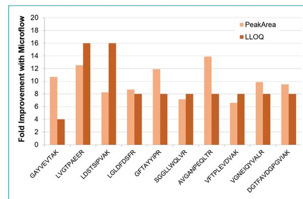
LLOQ gains and peak area improvements are shown for 10 synthetic peptides in diluted crashed plasma using microflow LC-MS at 3 µL/min vs. analytical flow LC-MS at 500 µL/min.
