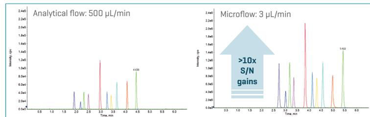
Peptide mix separation (500  $\mu\text{L}/\text{min}$ ) is shown with a 2.6  $\mu\text{m}$  C18 3 x 50 mm column and no matrix.
