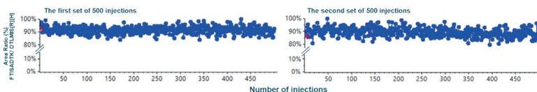
A 3.08% peak area ratio CV over 500 injections is shown with no increase in back pressure.
