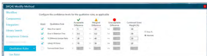
Figure 4b. Method editor in SCIEX OS software, user input for qualitative rules (traffic lights) to enable easy results review and filtering
