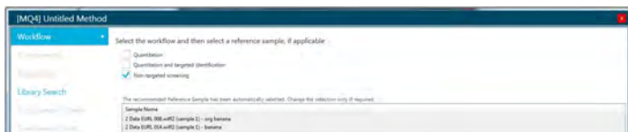
Figure 5a. Method editor in SCIEX OS software for unknown identification, selection of sample and control-sample for non-target peak finding
