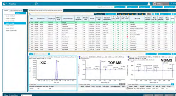
Figure 5b. Pesticides identified in proficiency test sample 2 in positive polarity based on matching retention time, accurate mass, isotope pattern and MS/MS library searching (note: Fipronil and Flubendiamide were identified in negative polarity)
