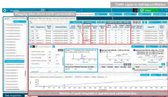
Figure 12. SCIEX OS Software Allows the Simultaneous Review of Qualitative and Quantitative Results
