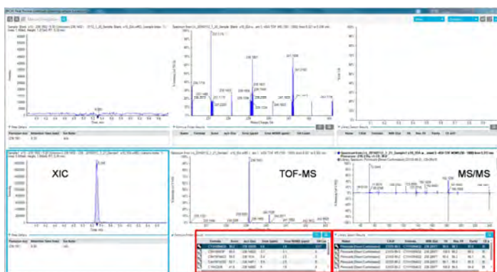
Figure 7a. Review of XIC of m/z 239.150 at RT 5.3 min and spectra with a found formula of C_{11}H_{18}N_4O_2
