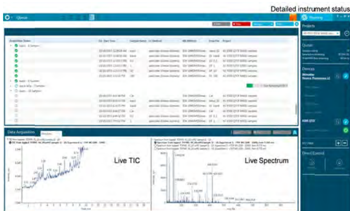
Figure 11. SCIEX OS Software Queue Manager with Inserted Auto-Cal Samples and Detailed Instrument Status Panel
