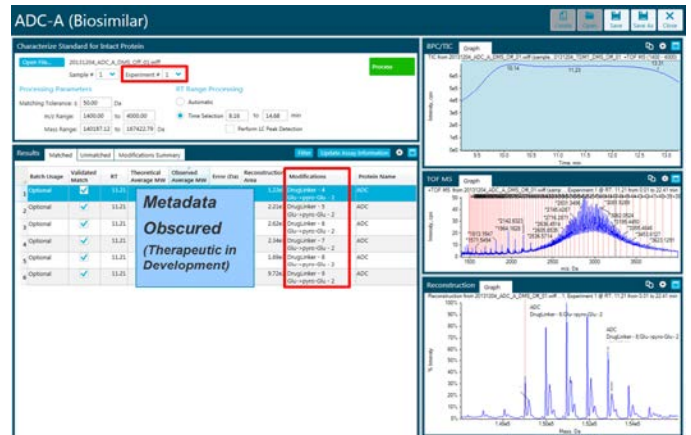
Figure 1: BioPharmaView(TM) software screenshot showing the panels relevant to the analysis. From left top clockwise: processing parameters, chromatogram, raw data, deconvoluted data, tabular summary.
