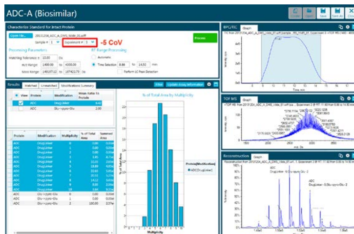
Figure 4: DAR table and distribution for an ADC molecule in development showing the utility of SelexION™ to revealing previously unseen species.
