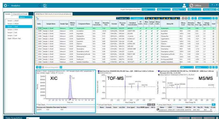
Figure 5a. Pesticides identified in proficiency test sample 1 in positive polarity based on matching retention time, accurate mass, isotope pattern and MS/MS library searching (note: Fludioxonil was identified in negative polarity)
