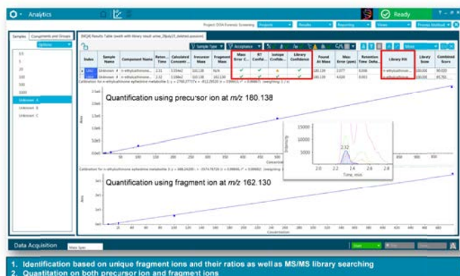
Figure 37. Identification and Quantification Results for n-Ethylcathinone Ephedrine Metabolite Compound Analysed by SWATH® Acquisition
