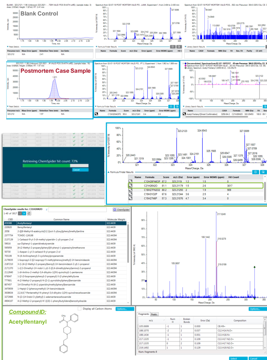
Figure 7. Consolidated Data Processing through SCIEX OS Software. A forensic postmortem blood sample analyzed using the SCIEX X500R QTOF System was automatically processed with a non-targeted screening workflow, which enabled the quick identification of Acetylfentanyl with high confidence in the ChemSpider search results. The in silico MS/MS spectral match further affirmed the finding of the fentanyl analog in this case.
